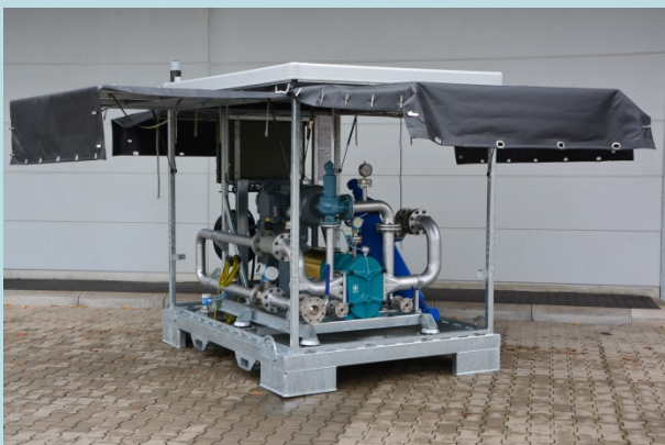
Tarp / roof bow construction with weather protection
