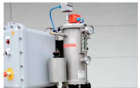
TS container with fill level monitoring, pressure protection, circulation pump and temperature monitoring of the barrier fluid
