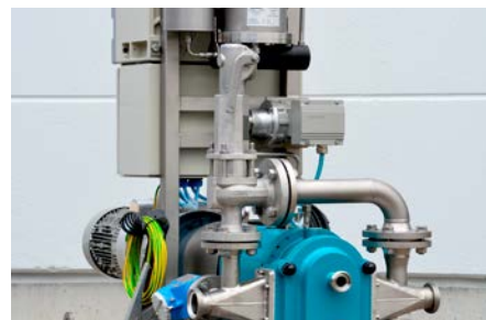
Overpressure protection by bypass with safety valve
