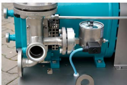
Electronic pressure measurement at suction and pressure side
