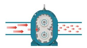
Time and again, impurities block pumps or even entire systems. As a result, time-consuming and cost-intensive maintenance work is required. The Multicrusher macerates impurities efficiently and reliably. For demanding macerating tasks, the Multicrusher is equipped with large inlet and outlet openings, so that even coarse solids can be macerated effectively and in an energy-efficient way.
